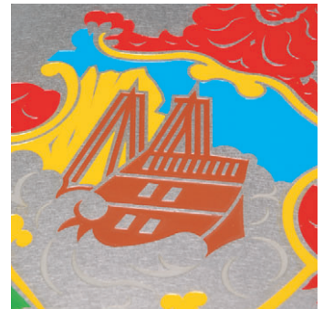
Waterjet cut, etched multi-coloured infilled st.stl. plate
