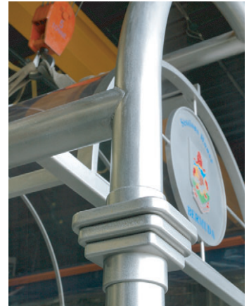
Suspended St. Stl. etched and infilled crest
