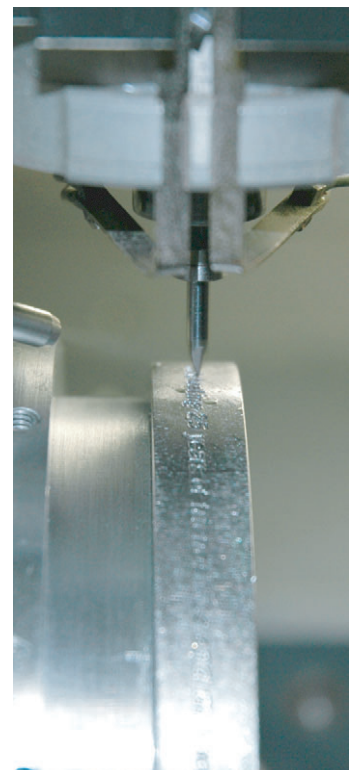
Live photo of CNC machining system on curved surface
